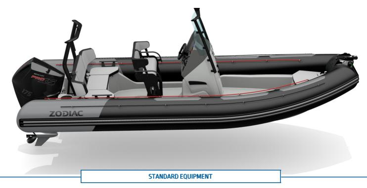
HULL & DECK: 1 Bow Bitt / 2 Aft Cleats , 1 Bow D Ring / 2 Towing Rings , 2 Bailers, 200L Integrated Tank, Fairleads, GRP Deep V-Hull, Lockable Mooring Storage, Self Bailing Countermoulded Deck (when empty), Ski & Wakeboard Locker, Tilting Console.
